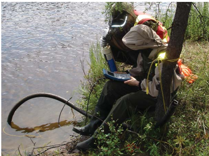
Environmental personnel deploy a real-time water quality instrument at Reid Brook
